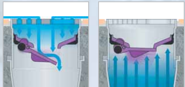
Multistop works without complicated technology simply according to the principle of gravity.
